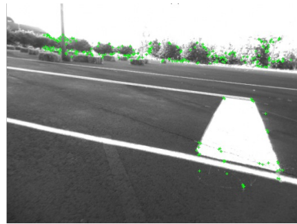
(b) Ground surface with low texture resulting in degenerate data.
